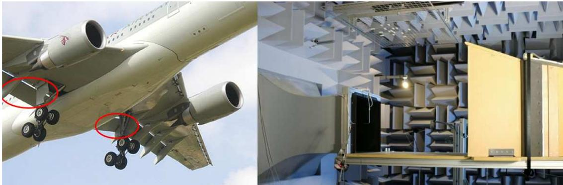
*Left : Landing airplane. The noise mechanism under investigation is the interaction of the gear wake with the flap (underlined in red). Right: the anechoic wind-tunnel at Institut PPRIME.*
