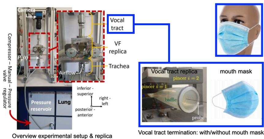
Fig 1: Overview of experimental setup and replica structure [1] and time-varying vocal tract [2] termination without/with mouth mask [3] to be studied.
